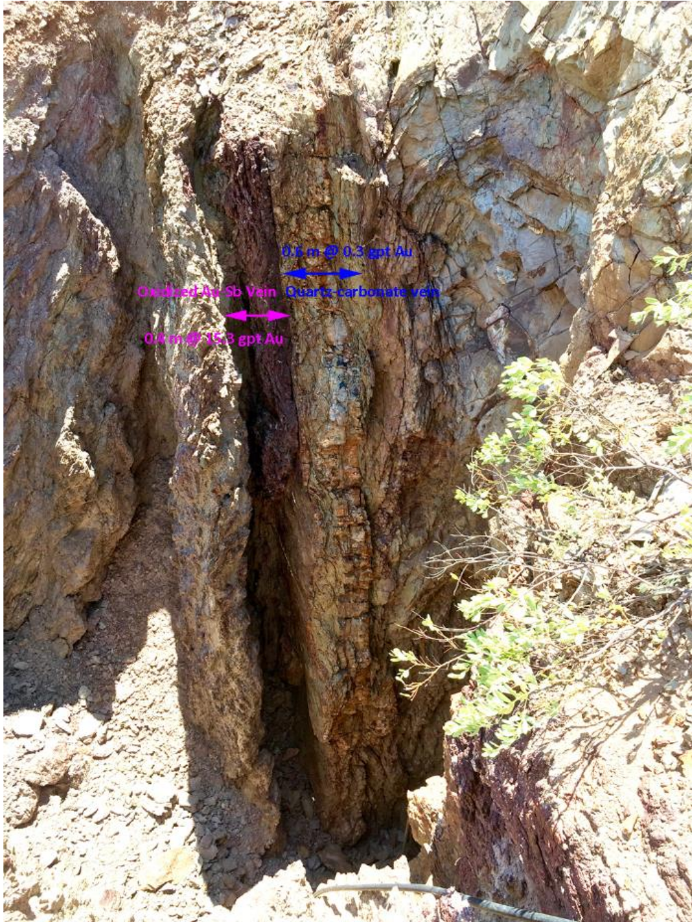
(Figure 1: Parallel gold-antimony and quartz-carbonate veins exposed in the wall of the collapsed historic Gold Spec shaft. The gold-antimony vein contains 15.3 gpt Au, is heavily oxidized, and is primarily composed of iron and antimony oxides and minor quartz. This type of vein is soft and weathers recessively making exposures uncommon and surface exploration challenging. The neighboring quartz-carbonate vein carries only 0.3 gpt Au, but is more resistant to weathering. It is common to find such vein material at surface, but it usually does not contain high gold grades.)
