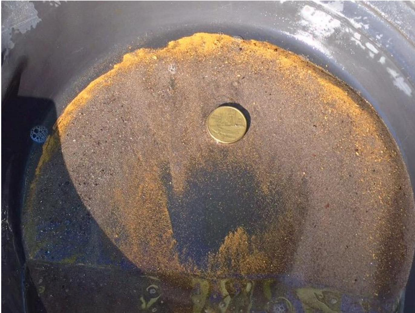
*(Figure 2: Very fine to medium gold grains from concentrate produced during commissioning test work on the IGR3000 gold recovery plant. The coin is approximately 1.5 cm across.)*
