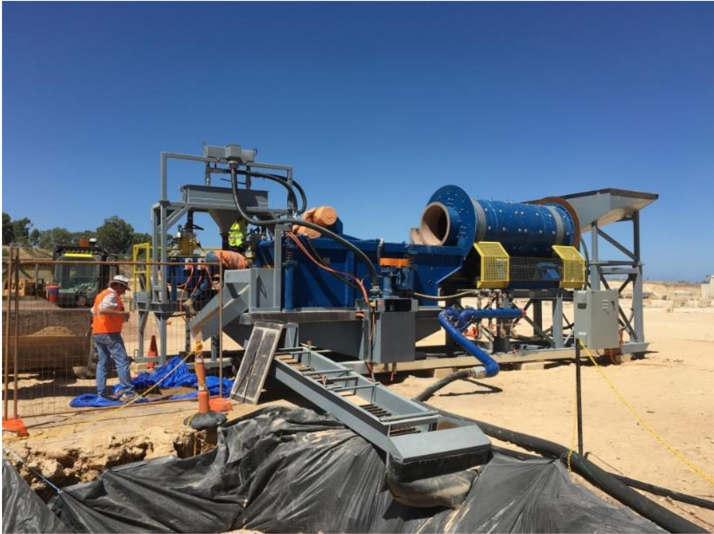
*(Figure 1: Novo's IGR3000 gold recovery plant being commissioned at a gravel quarry near Perth.)*
