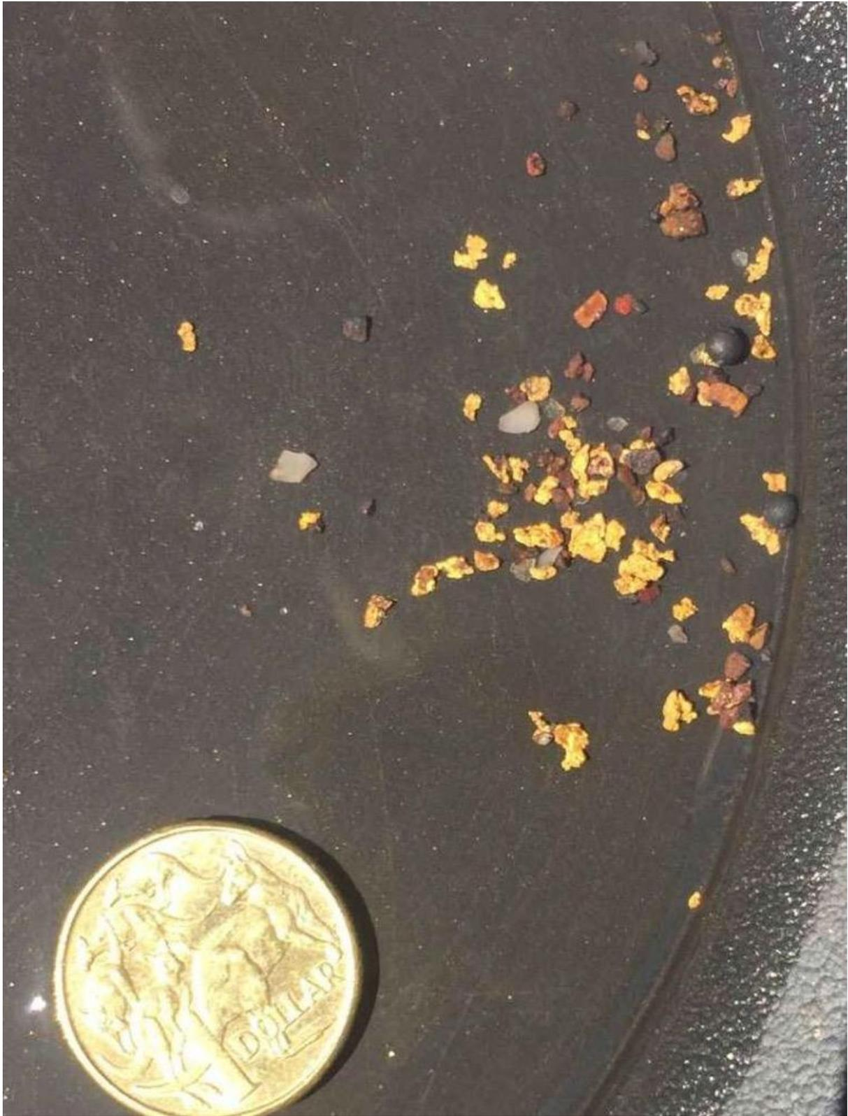
*(Figure 3: Coarse gold grains up to 4 mm across collected from concentrate produced during commissioning test work on the IGR3000 gold recovery plant. The coin is approximately 2.5 cm across.)*
