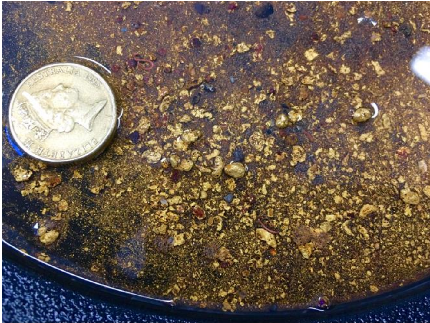
(Figure 5: Coarse grained Au recovered from RM100GO! pulverized product and separated using the IGR 3000.)
