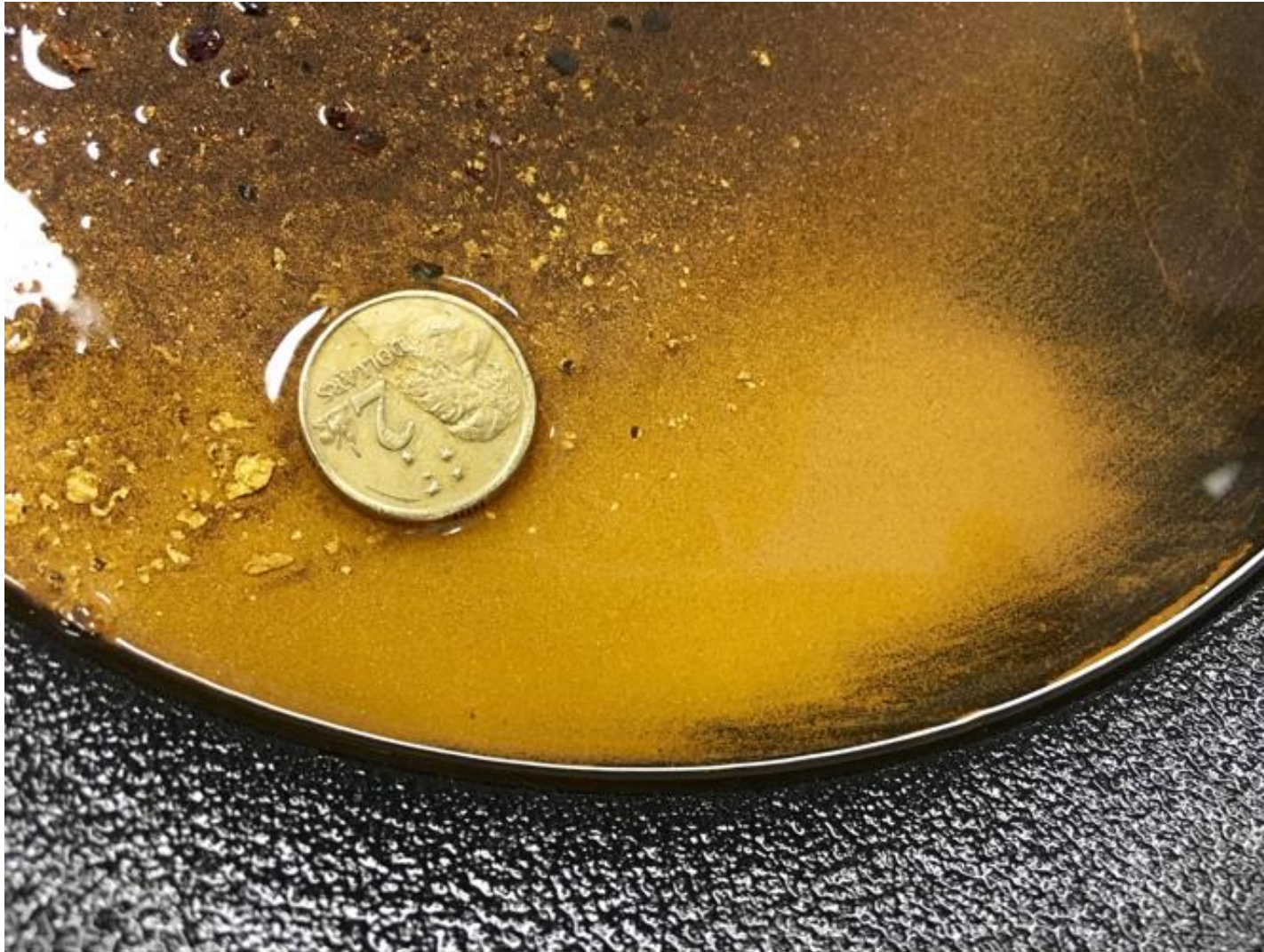
(Figure 4: Fine grained Au recovered from RM100GO! pulverized product and separated using the IGR 3000.)
