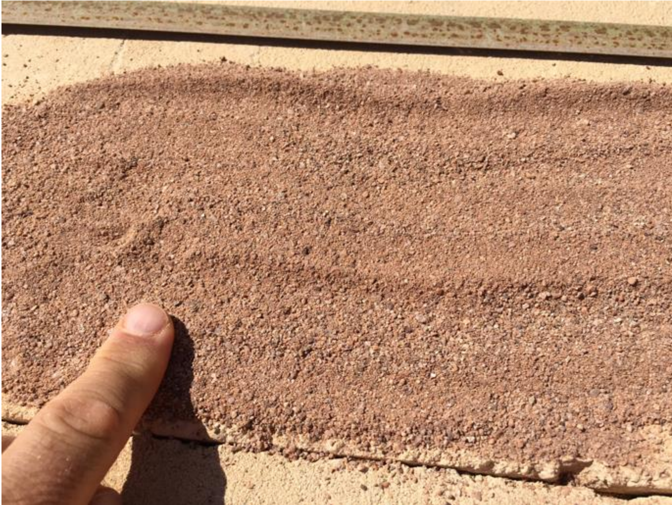
(Figure 3: Close up of pulverized rock produced by the Rubble Master RM100GO! Impactor. Initial screen tests indicate a crush size of P80 -1 mm.)
