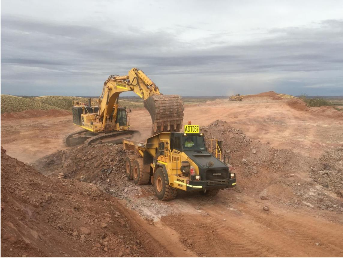
*(Figure 2: First load of mineralized conglomerate being loaded into an articulated truck. The flat area in the background is pre-stripped of waste. The D9 bulldozer in the far distance is removing the final waste material.)*
