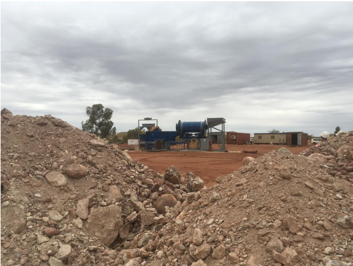
(Figure 1: Novo’s IGR3000 trial processing plant installed at Beatons Creek. Mineralized conglomerate stockpiles in the foreground.)
