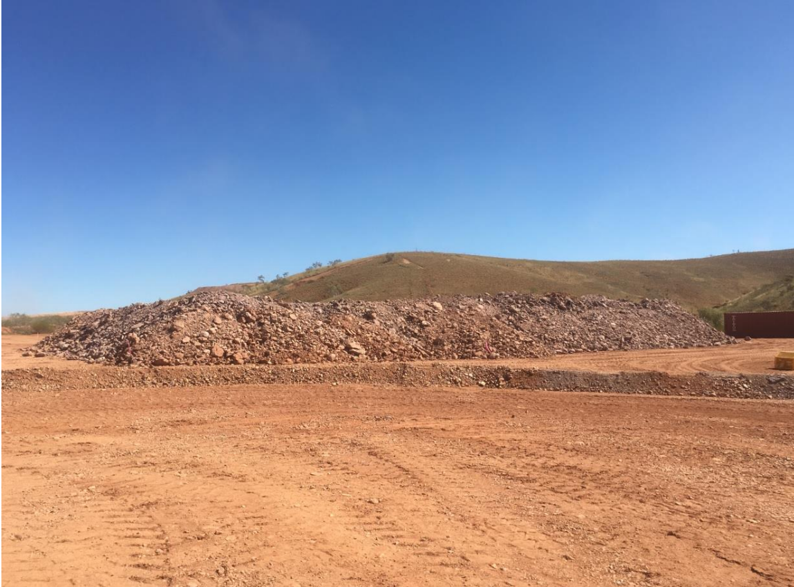
(Figure 2: Stockpile of mineralized conglomerate bulk sample on the run-of-mine pad. Processing of this material will commence within a couple weeks.)
