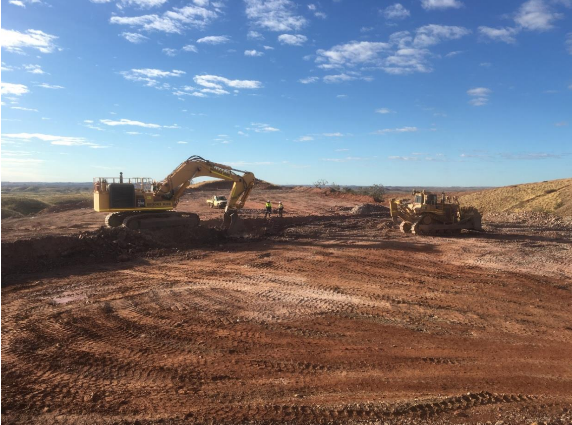
(Figure 1: Bulk sampling a bench of mineralized conglomerate. The excavator sits atop the conglomerate. Note the good continuity of this horizon across the pit floor.)
