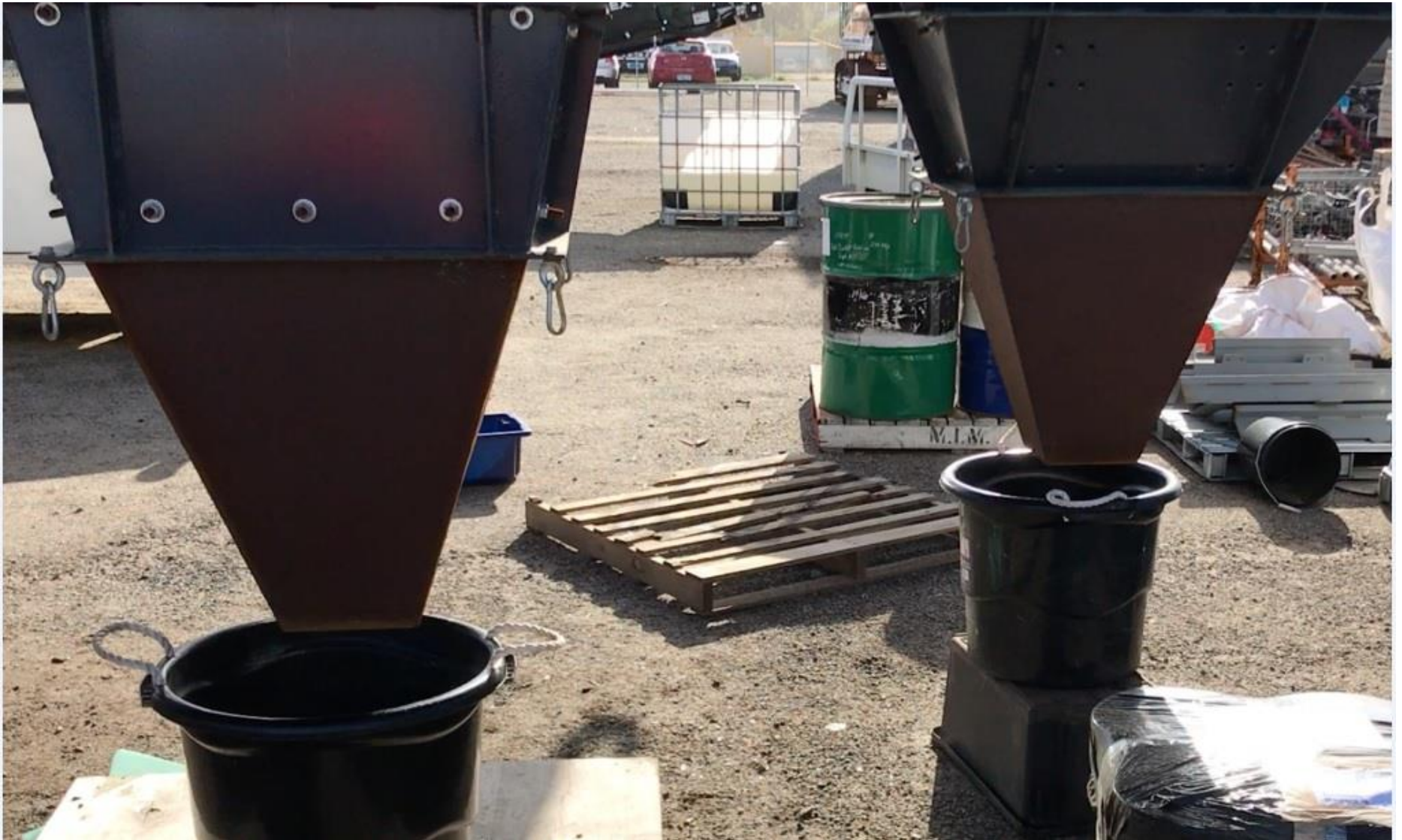
(Figure 2: Discharge shoots of Steinert XSS T sorting machine. The shoot on the left collected rock particles with no detectable coarse gold, “ Sorted Tailings, ” and the shoot on the right collected rock particles containing coarse gold particles, “ Sorted Concentrate. ”)
