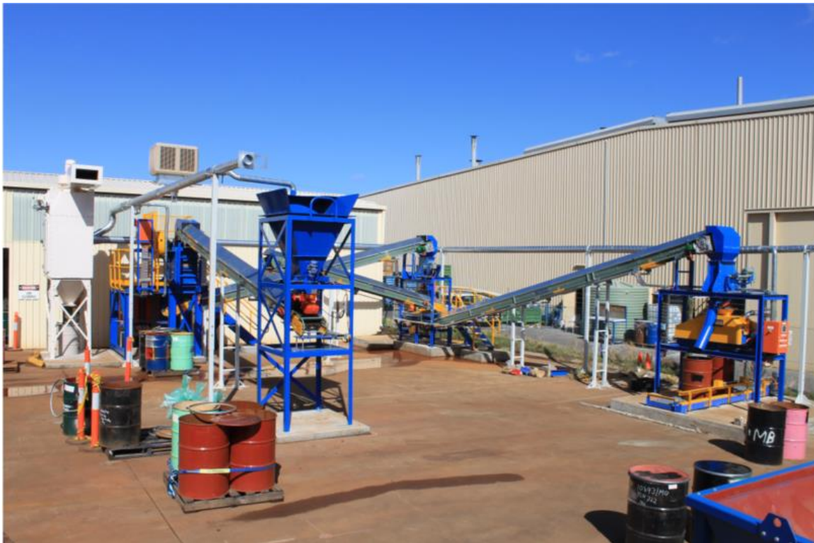
(Figure 1: Comminution circuit of the SGS test plant. It is anticipated that 3-4 5-tonne bulk samples can be processed per week by this facility. Bulk sample test work will be overseen by the existing scrutineering regime ensuring sample integrity in a certified laboratory environment.)
