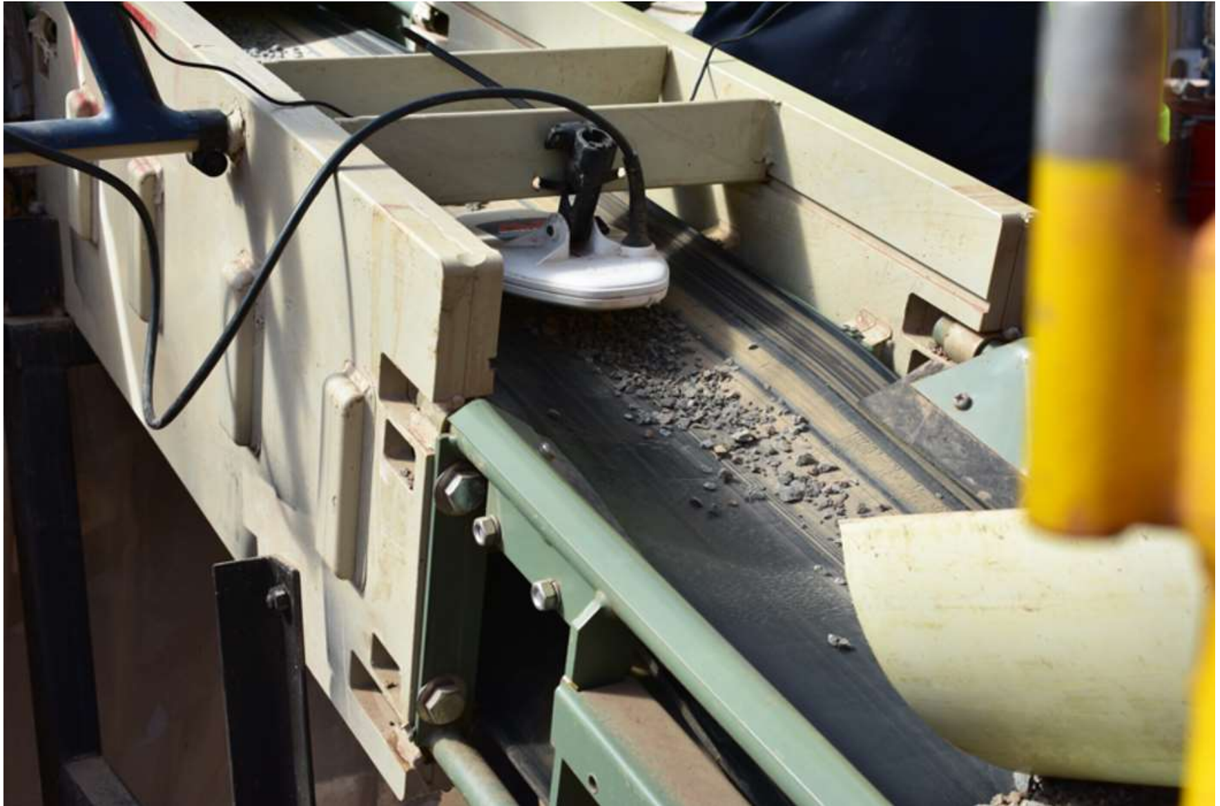
(Figure 1: A metal detector fitted to a conveyor is used to isolate coarse gold nuggets from crushed rock at SGS Minerals, Perth.)
