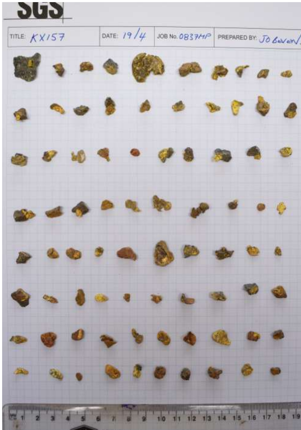
(Figure 2: The above gold nuggets, some partially encased in rock matrix, were recovered from a 7,143 kg bulk sample, KX157, from Comet Well. Blue gridlines are 5 mm. Nuggets range in size from about 3 mm to 2 cm. In spite of two stages of crushing, most appear intact and relatively unscathed retaining their characteristic flattened melon seed appearance, a clear indication of a water-worn alluvial origin. Fine-grained “halo” gold particles are observed around nuggets partially encased in rock matrix similar to that observed around nuggets recovered from Purdy’s Reward.)
