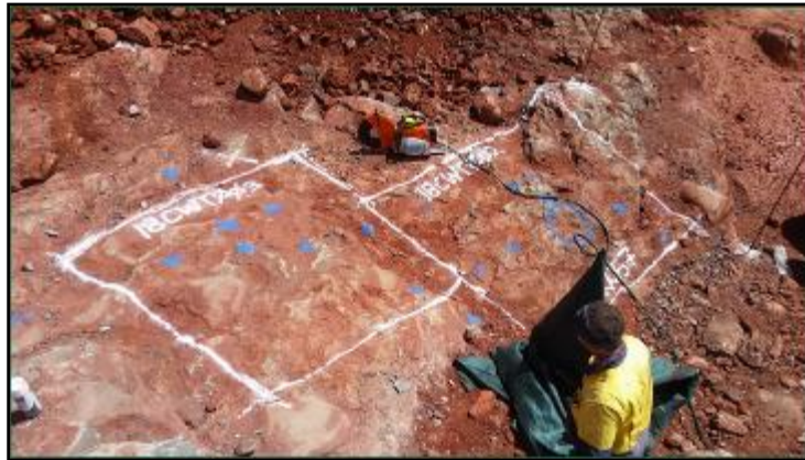
Figure 11.7 Bulk Lateral Sampling practice: Sample mark out (top), rock breaking a sample with a fly rock screen (centre), final sample location surveyed in 3D and photographed (bottom)
