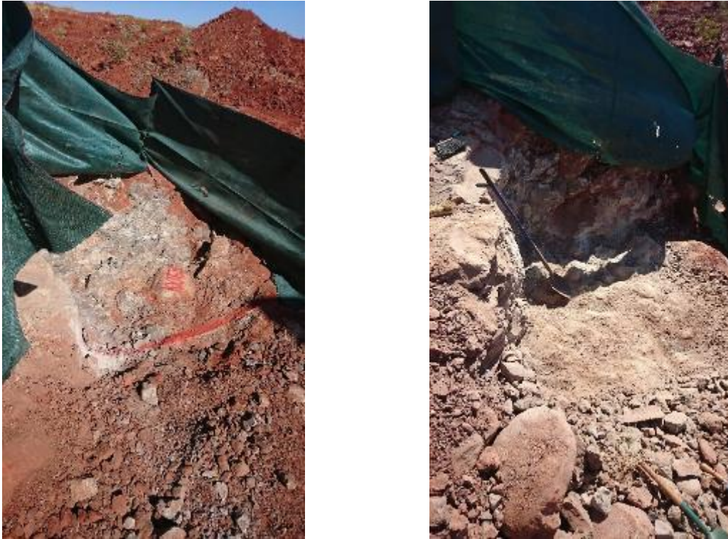
Figure 10.6 Example of bulk sampling protocol for sample KX153 pre (left) and post (right) collection
