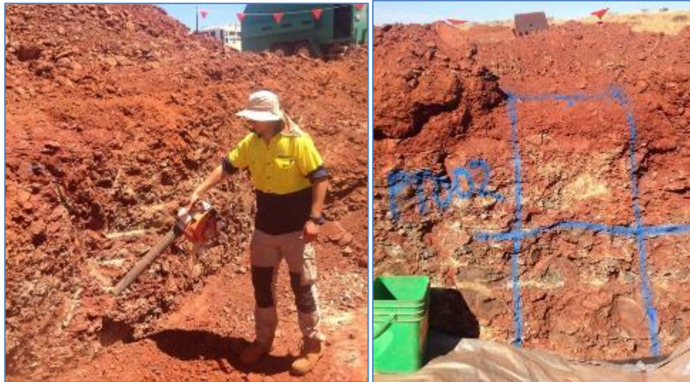
Figure 11.3 Sampling using a jack hammer (left) and transferring fines (right)
