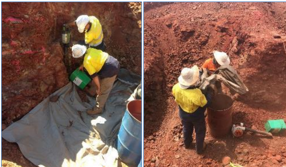
Figure 11.3 Sampling using a jack hammer (left) and transferring fines (right)
