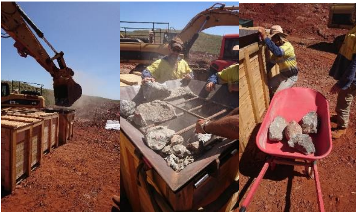
Figure 10.7 Bulk sample collection for Karratha samples. Wooden crates and a metal hopper with a grizzly were used to allow larger rocks to be captured and broken for the sample.
