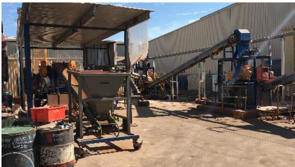
Figure 11.9 SGS pilot plant front-end crushing circuit
