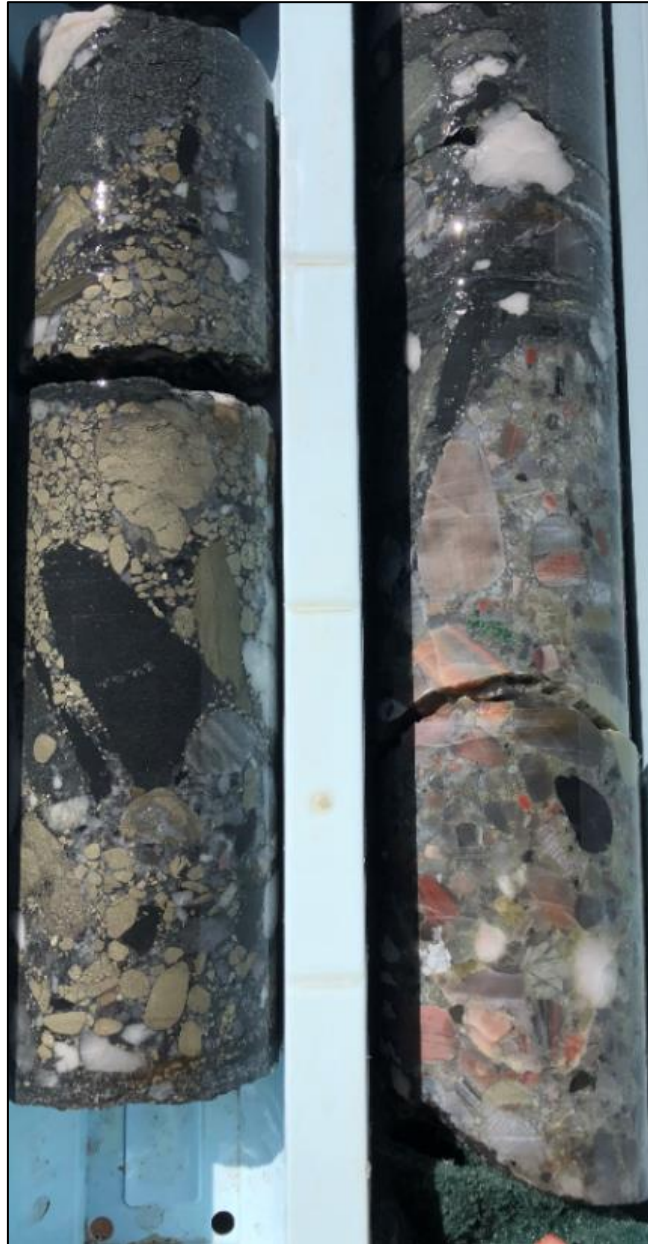
Figure 7.12 Detrital pyrite and dromedary boulder (bottom right) in 2018 PQ drill fresh mineralised core (85 mm diameter)
