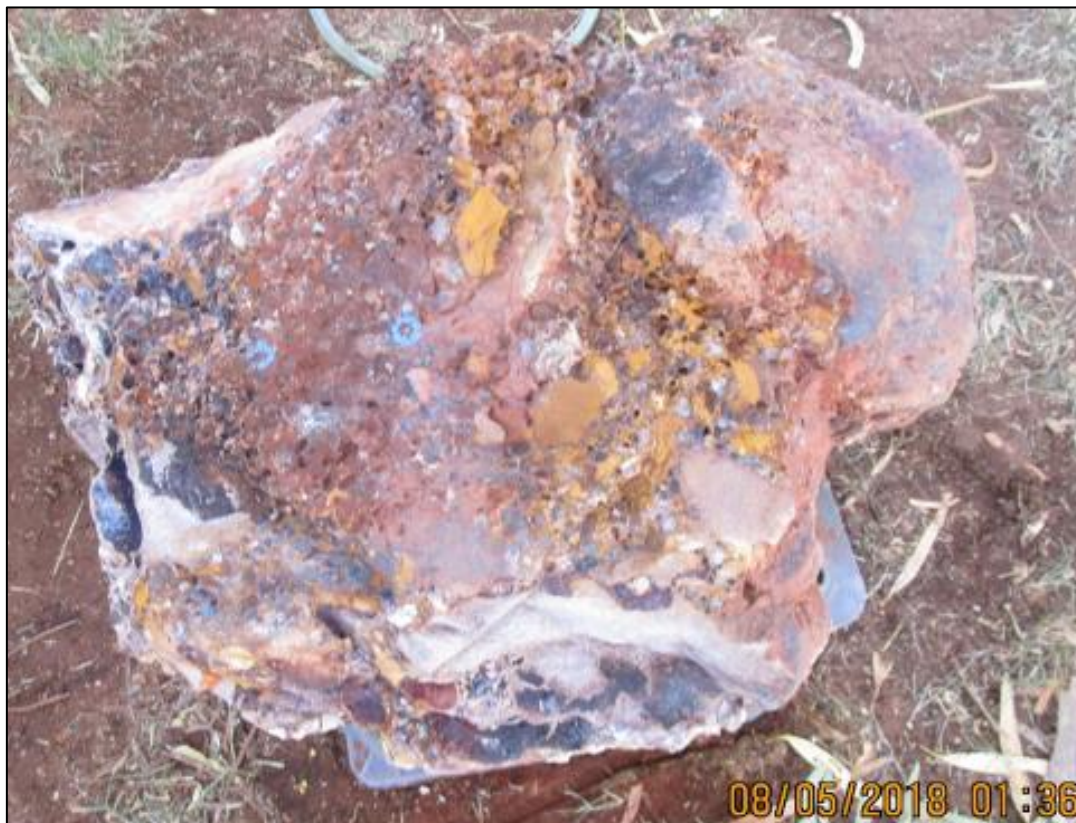
Figure 7.6 Gold particles shown within blue circles amongst buckshot pyrite (black dots) from a ferruginous channel conglomerate (South Hill area)
