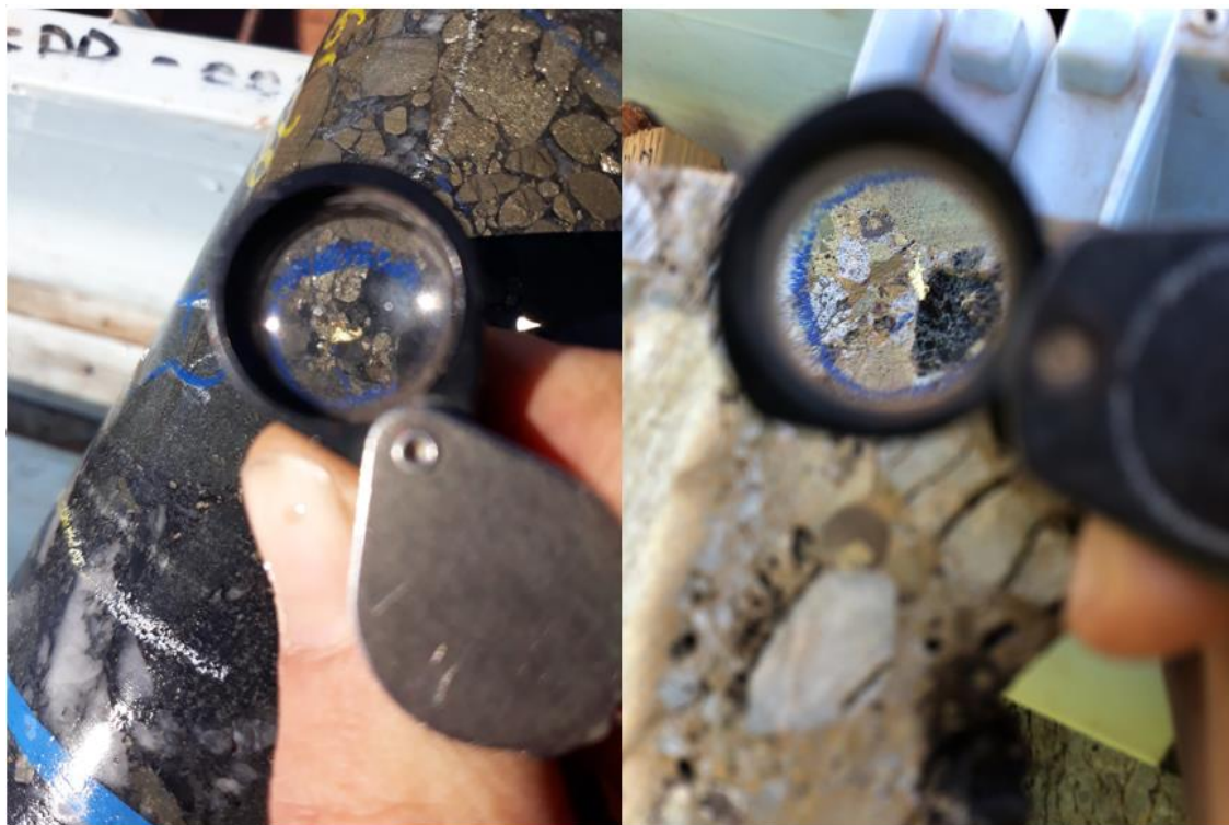
Figure 7.7 Gold in drill core (left: BCDD18-002, 60.8 to 61.3 m, 7.3 g/t gold and right, BCDD18-001, 6.12 to 6.6 m, 4.3 g/t gold)
