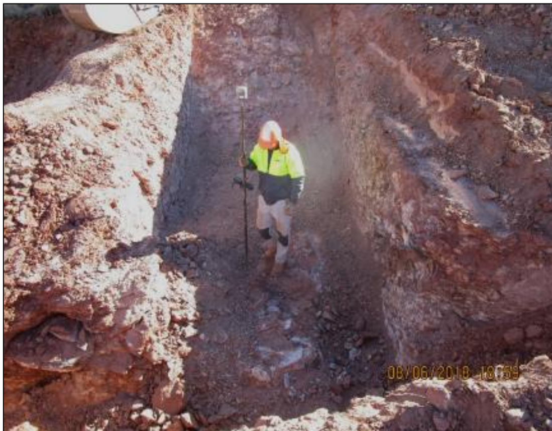
Figure 9.1 Measuring a trench bulk sample
