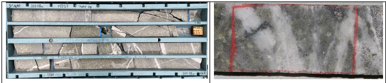
(Figure 3: Strongly sericite altered and quartz veined interval of Missing Link Monzogranite from 261.08 m – 264.78 m in MD17. Right photo is close-up of drill core from 263.4 m – 263.5 m. The enveloping one metre interval (263 m – 264 m) returned 1.24 ppm Au, 145 ppm Sb, 2.01 ppm Ag, 5530 ppm As (0.55%), 20 ppm Bi, 30 ppm Mo, and 439 ppm W.)
