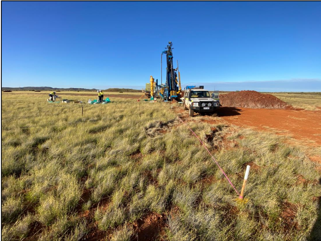
Figure 2: Field photo of the Stark Drilling RC rig at Morto Lago.
