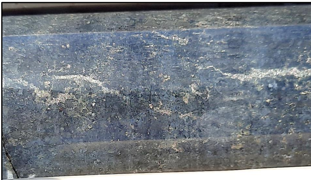
Figure 3: Hole KD902 at approximately 103.52 m, showing disseminated and stringer sulphides. Spot assays of sulphide with pXRF yielded 0.79% Ni and 0.21% Cu.
