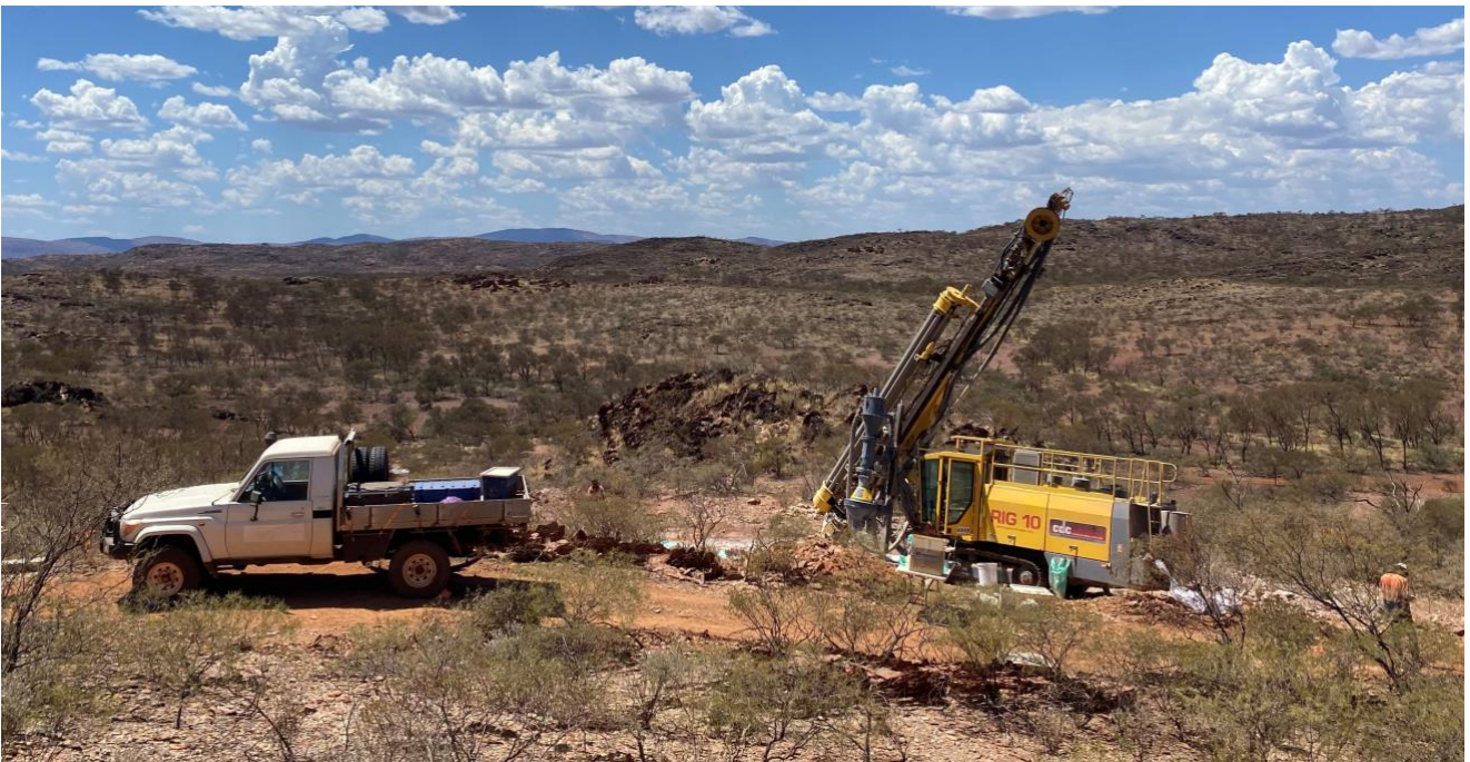
Image 1 Reverse Circulation drilling at the Catia prospect at the Bellary Dome Project, March 2023
