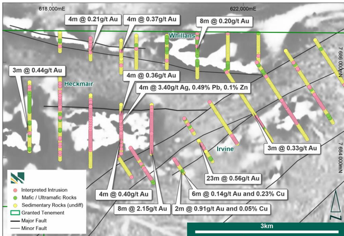
Becher target area showing peak gold assays, results from lithogeochemical assessment draped over 1VD aeromagnetics.
