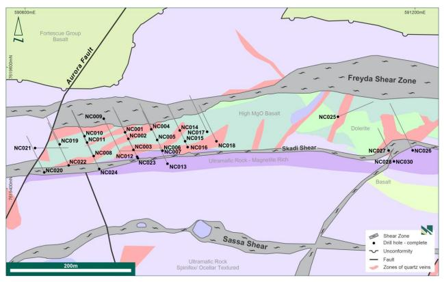
Figure 3: Nunyerry North geological interpretation and drill hole location plan.
