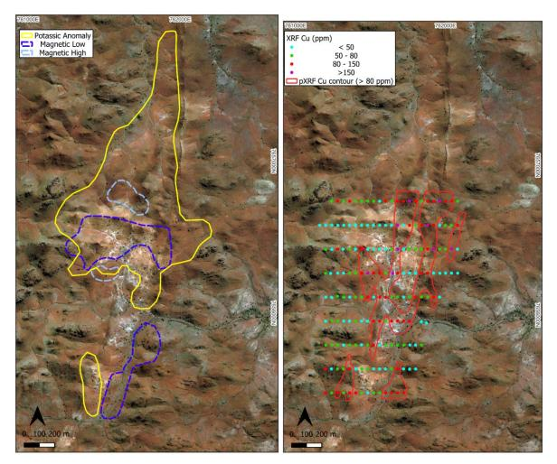
Figure 7: Shady Camp West highlighting geophysical anomalies (left) and pXRF soil Cu geochemical anomalies (right). The potassic anomaly over 2.2 km strike partially overlaps with intense clay alteration of porphyries and host basalt (light colouration on the imagery). Coherent Cu anomalism is open and untested to the north and correlates with maximum quartz veining and weak Au and Mo anomalism in soils.
