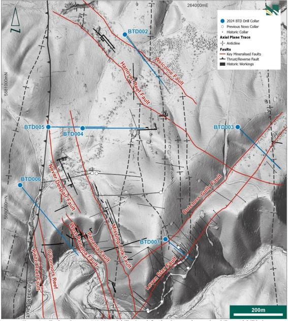
Figure 6: Collar location map (LIDAR) and drill azimuth for the six recently completed diamond drill hole at Belltopper. Key structural elements and target mineralised reefs (red lines) also delineated.
