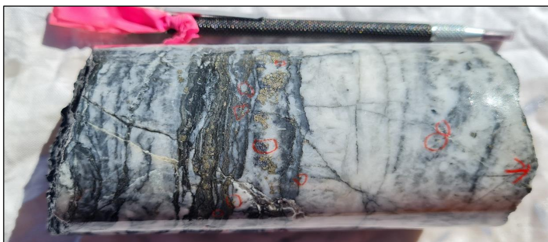
Figure 10: Diamond drill core from NBD005 displaying visible gold 18 (red circles) in a laminated quartz vein at a depth of approx. 97 m. Refer to significant diamond drilling results in Appendix 5.
